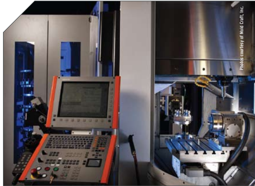
Robotic interface to simultaneous four-axis CNC.
